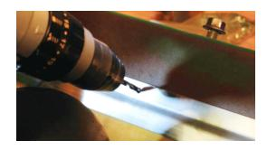
5. Hold the strip in position, working from the center outward, drill and rivet one hole at a time. Be sure to install each rivet before moving on to the next hold. If you do not have a rivet gun capable of pulling 3/16 steel rivets you many use the self drilling screws in place of rivets. Both are provided for your convenience.
