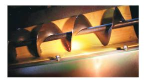
Note: It is important that there is sufficient clearance approximately 1/8" between the auger and the liner. You may need to loosen the bolts on the rear bearing mount to even the clearance between the two troughs. Also, notice we removed the crop dividers for extra room during installation.
